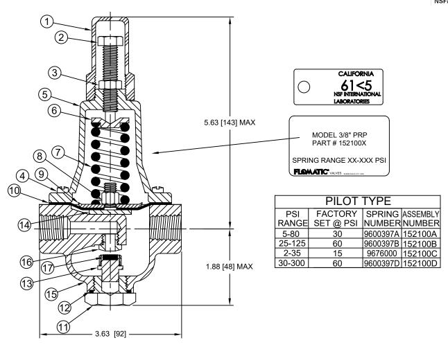
Max Temp 180°F (82°C) Max Pressure 400psi (28bar)
