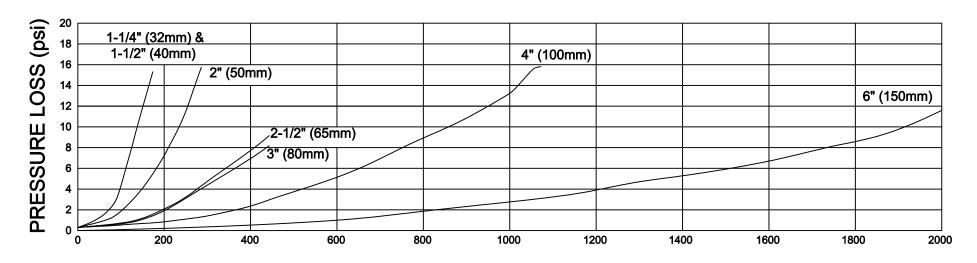
FLOW RATE (gpm)
